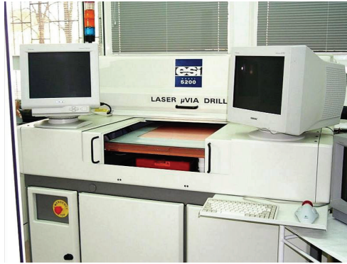
Fig. 1. A view of the ESI 5200 laser \mu\text{via} drill
