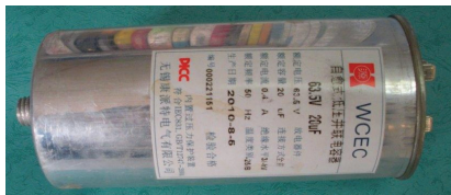
Fig.3. The C_3 used to harmonic voltage measurements
