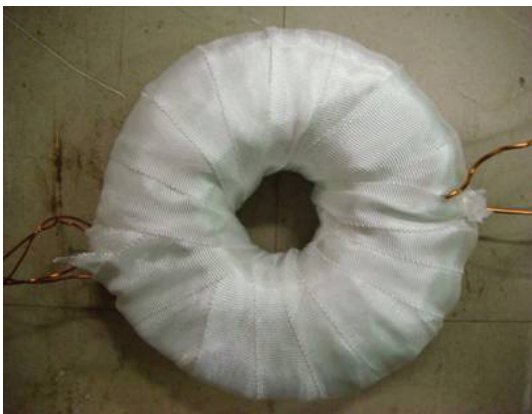
Fig.2. Ring sample for measurement at high temperature.
