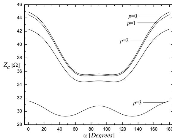
Fig. 5 – Variation of the characteristic impedance with rotation angle and eccentricity when  $c/d=0.5$ ,  $a/d=0.2$ ,  $b/d=0.3$ ,  $s=0.5$ .
