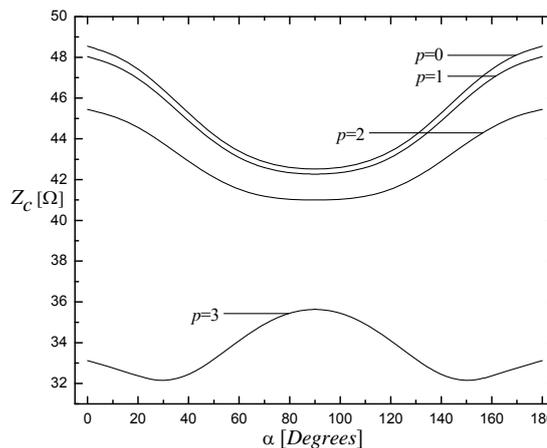
Fig. 4 – Variation of the characteristic impedance with rotation angle and eccentricity when  $c/d=0.5$ ,  $a/d=0.2$ ,  $b/d=0.3$ ,  $s=0$ .
