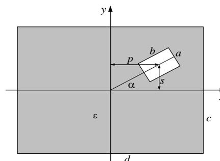
Fig.1. Double eccentric rectangular coaxial line with rotated inner conductor
