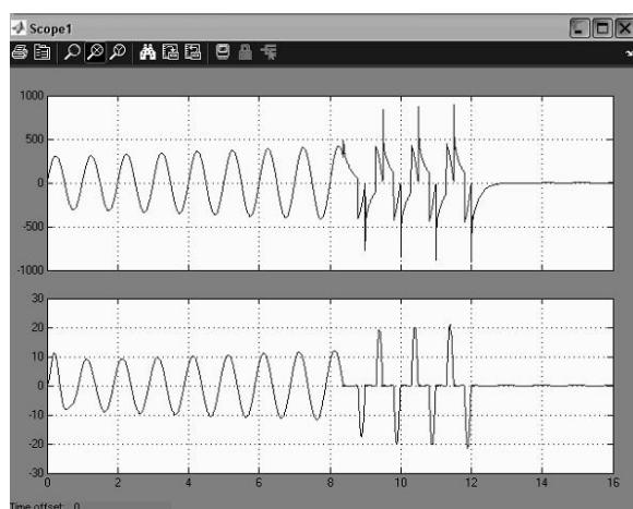
Fig. 2. The simulation results of RLC load cut off at voltage increase
