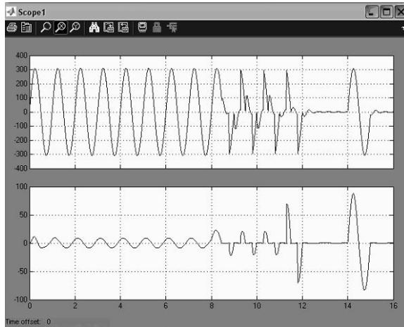
Fig. 3. The simulation results of RLC load cut off at current increase
