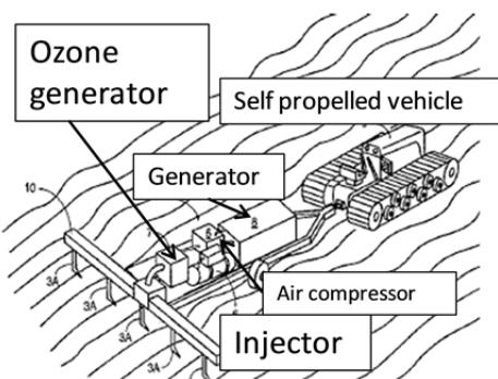
Fig.2. Field sterilization (US Pt. 5624635)
