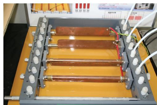
Fig.1. The 12 channel DBD electrode system
