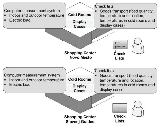
Fig. 3. Parameters and electric load measurements
