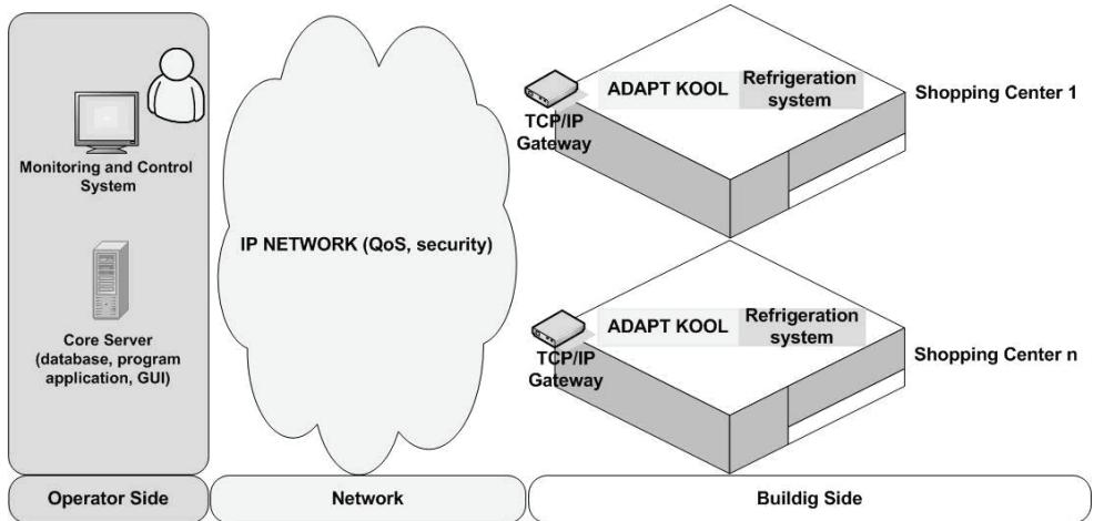
Fig. 6: The architecture of real-time EMS
