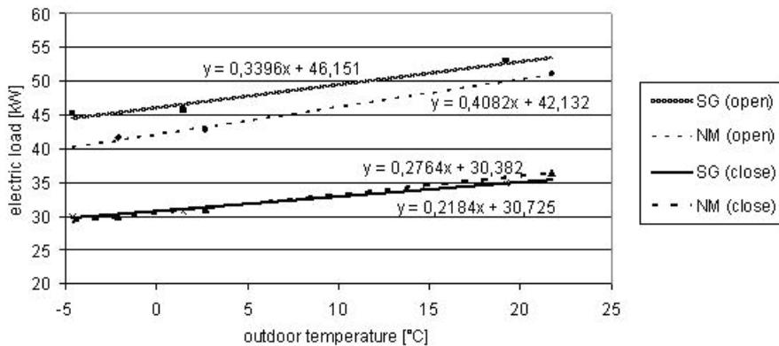
Fig. 5: Approximation functions presenting the relationship between the electric load and outdoor temperatures
