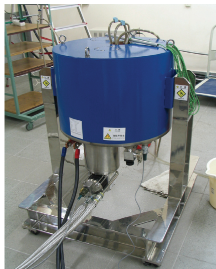
Fig. 12. View of LTS electromagnet as a source of magnetic field for experimental system
