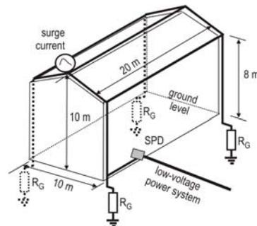
Fig. 3. Diagram of lightning protection systems (case B and C)
