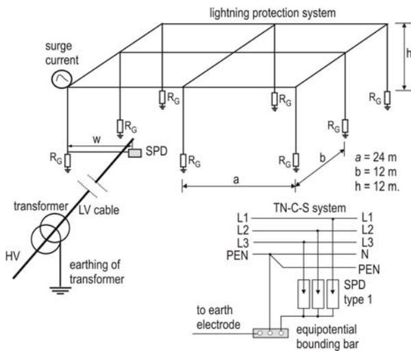
Fig. 2. Model of LPS and LVPS used in calculation (case A)
