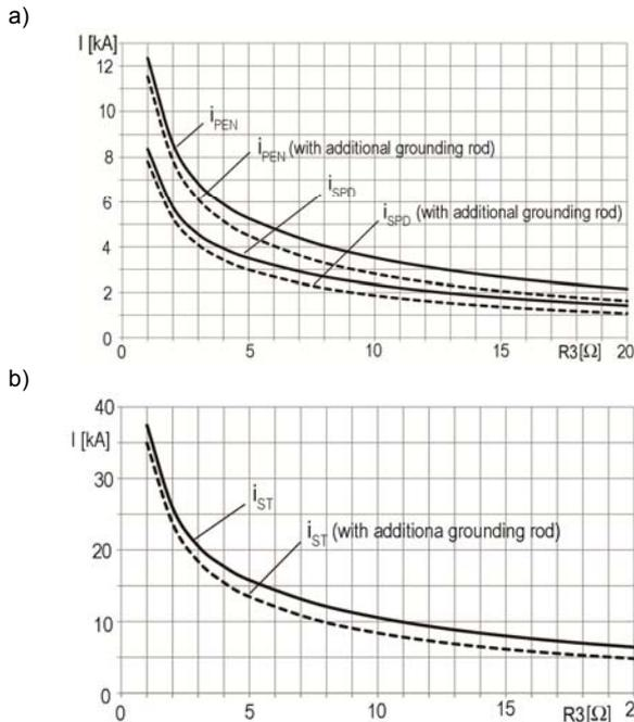
Fig. 5. Maximal values of currents with increasing values of transformer grounding system (case A,  $d = 100$  m,  $w = 2$  m), a) currents in SPD and in PEN conductors, b) total current in LVPS
