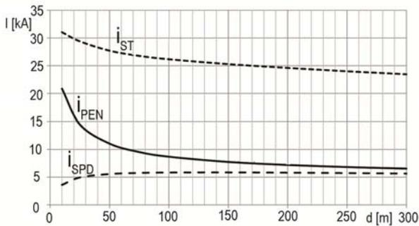
Fig. 6. Maximal values of currents in conductors of LVPS (case A,  $w = 2$  m) with increasing distance  $d$  between SPD and transformer
