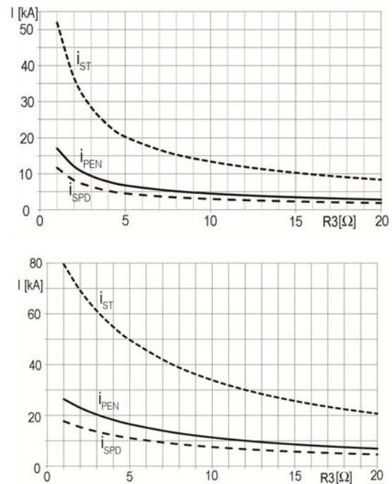
Fig. 7. Maximal values of currents in conductors of LVPS with increasing values of transformer grounding system ( $d = 100$  m,  $w = 5$  m., a) office building - case C, b) residential building - case C
