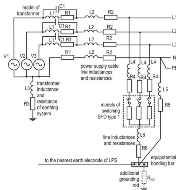
Fig.1. Circuit diagram for LPS with switching SPD type 1
