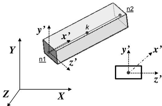
Fig.2. Coordinate systems: global (XYZ) and local ( $x'y'z'$ ) used for  $k$ -th element having two nodes (n1, n2)
