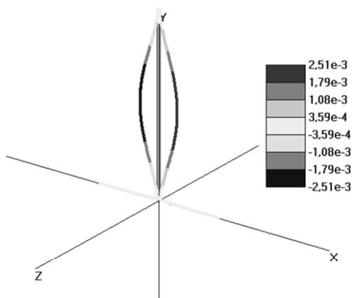
Fig.6. The calculated displacement  $U_x$  [m], of the circuit under study. Scale exaggerated. 150 Finite Elements used
