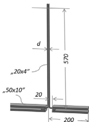
Fig.5. The test circuit used for measurements, which validated the proposed calculation method ( $d = 4\text{mm}$ , air-gap between beams)
