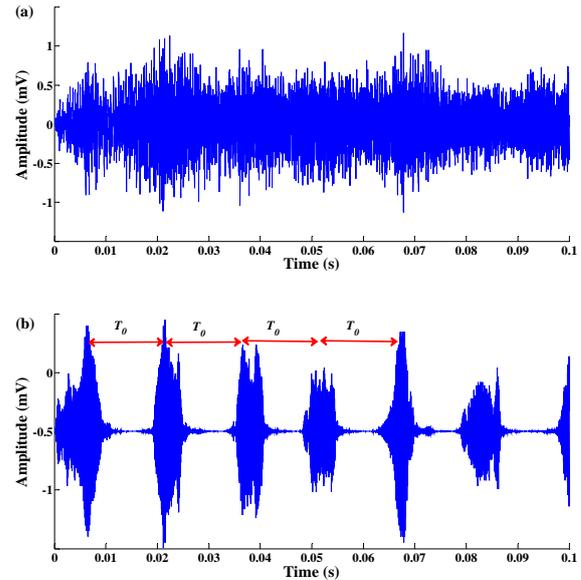
Fig. 4. The time spectra: (a) original vibration signal and (b) NICA separated source.
