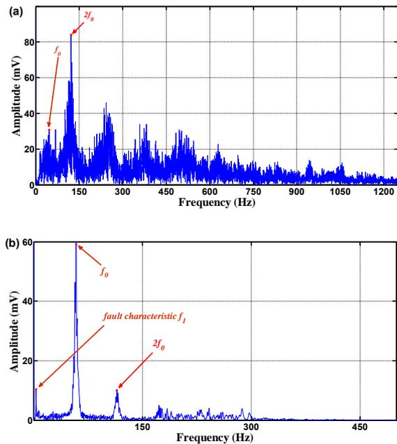
Fig. 5. The frequency spectra: (a) original vibration signal and (b) NICA separated source.
