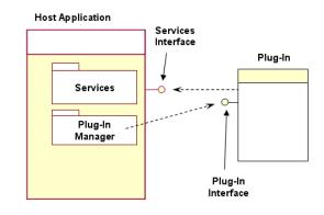
Fig.4 The example plug-in framework
