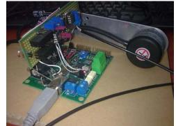
Fig.3. Electronic synchronization module with for IR camera
