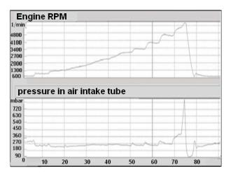
Fig.7. The speed and intake pressure at very slow opening throttle
