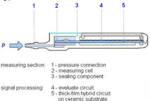
Fig.2. Thick film pressure sensor
