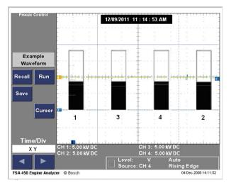
Fig.10. Graph of secondary voltage at higher revs
