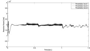
Fig. 7. Utility grid1 reactive power at bus 1.
