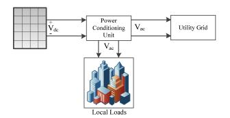
Fig. 1 Simplified diagram of the grid-connected PV system.
