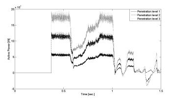
Fig. 5. Injected power by PV system at bus 11.
