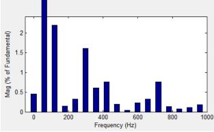
Fig. 16. Current harmonic spectrum at bus 11.
