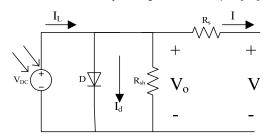
Fig. 2. Equivalent circuit of the PV module.
