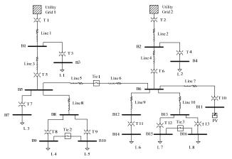
Fig. 3. Single-line diagram of the 16-bus test system.
