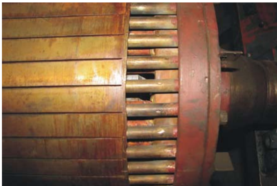
Fig.6. Fragment of modified rotor of 515 kW motor after 25 years of operation
