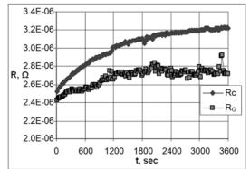
Fig. 3 Contact resistances,  $R_c$  of the classical and  $R_G$  of the G-design case copper connections as a function of time (for 1 hour)
