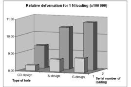
Fig. 11. Relative deformation (x 100 000) for initiating a force of 1N for the different hole designs when a different loading sequence is followed
