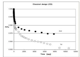
Fig. 4. Influence of the loading sequence (1<sup>st</sup> and 2<sup>nd</sup>) on the type of the relaxation curve for the case of simple hole (CD - classical design)
