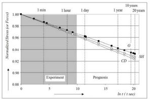
Fig. 10. Normalized stress relaxation of the design concept CD, S, and G after the second loading  $% \left( {{\rm{D}}_{\rm{A}}} \right) = {{\rm{D}}_{\rm{A}}} \right)$
