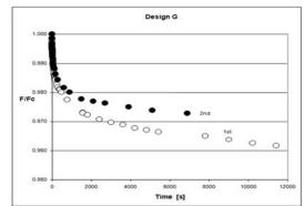
Fig. 6. Influence of the loading sequence (1<sup>st</sup> and 2<sup>nd</sup>) on the type of the relaxation curve for the case of bolt hole with groups of small holes (G-design)
