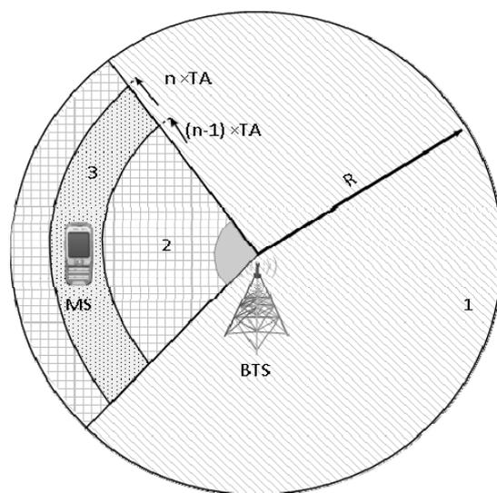
Fig.1. Basic localization method in GSM network
