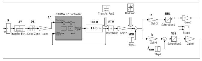
Fig.2. Structural chart of the ARS digital model of EAF-200 arcs lengths
