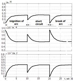
Fig.4. Time dependencies  $l_a(t)$ ,  $I_a(t)$  and  $U_a(t)$  ARS EM with a neuro-controller
