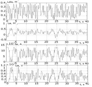
5. Time dependencies  $l_{dis}(t)$ ,  $l_a(t)$ ,  $I_a(t)$  and  $U_a(t)$  of ARS EM on the base of AFAR-T-12 controller under the influences of occasional disturbances
