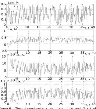
Figure 6 – Time dependencies  $l_{dis}(t)$ ,  $l_a(t)$ ,  $I_a(t)$  and  $U_a(t)$  of the designed ARS EM with a neuro-controller under the influence of occasional disturbances
