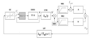
Fig.1. EAF power controller with a neuro-controller functional chart for one phase
