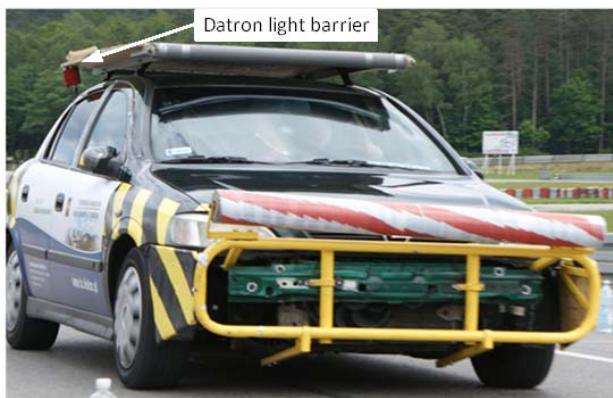
Fig. 6. Opel Astra research vehicle with attached front tubing and a photocell (light barrier)
