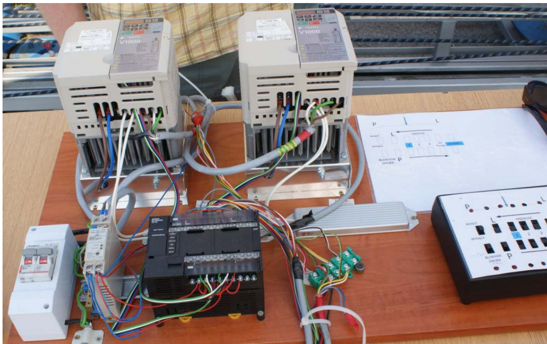
Fig.10. View of programmable system controlling the movement of mock-ups
