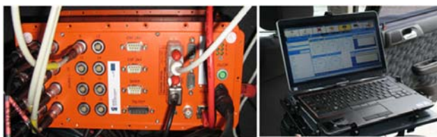
Fig.7 Data acquisition station with a tablet and ARMS software installed
