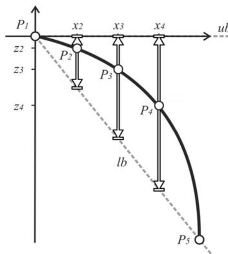
Fig. 2 The reflector profile (version 1); the illustration of limiting conditions of the permissible positions of interpolation nodes (points  $P_2, P_3, P_4$ )
