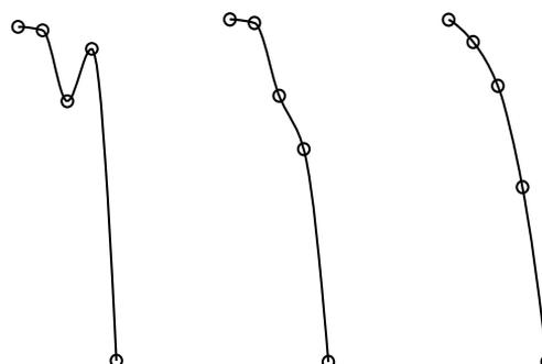
Fig. 6 The examples of the reflector profile curves generated in successive iterations of the unlimited optimisation process (from the left): the 3rd, 10th and 50th iteration; the circles mark the positions of interpolation nodes
