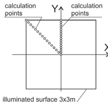
Fig. 5 The positions of 31 calculation points on the illuminated surface
