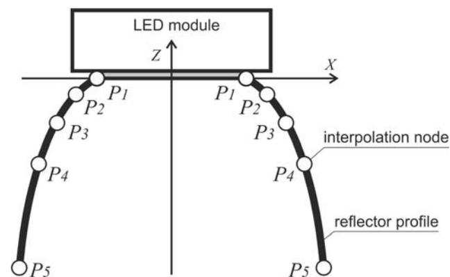
Fig. 1 The reflector model: LED module (light source),  $P_1, P_2, P_3, P_4, P_5$  – interpolation nodes
