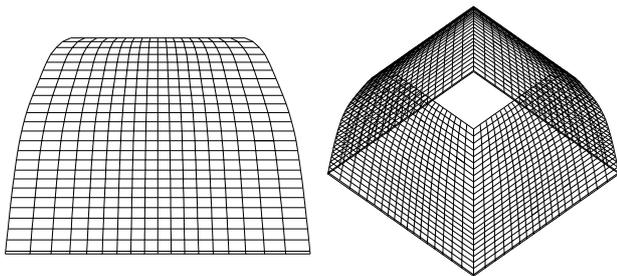
Fig. 4 The figure of the reflector model made of flat elementary surfaces. Side view and isometric view
