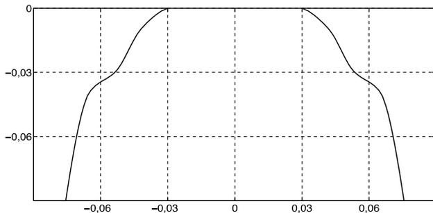
Fig. 8 The figure of a tri-curve reflector profile calculated with the algorithm without constraints
