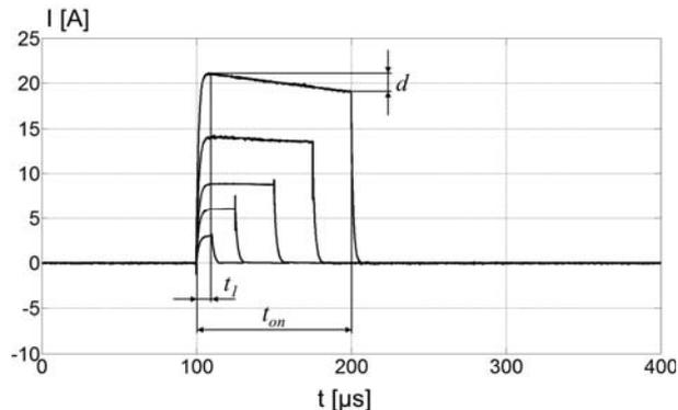
Fig.4. Examples of waveforms of pulse current ( $t_1$  - time to peak of amplitude pulse current,  $t_{on}$  - duration of pulse current,  $d$  - drop of pulse current)
