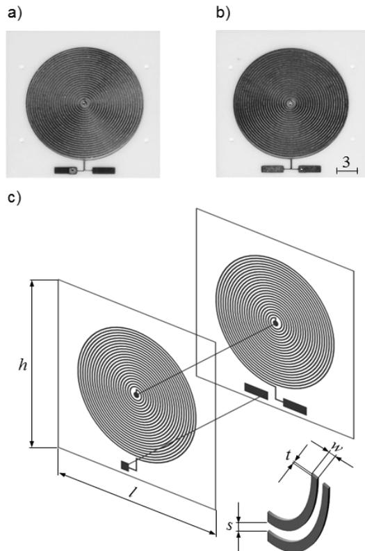
Fig.2. Test coil: a) photo of the top side, b) photo of the bottom side, c) schematic view ( $h = 20$  mm,  $l = 20$  mm,  $s = 0.15$  mm,  $t = 35$   $\mu\text{m}$ ,  $w = 0.15$  mm)
