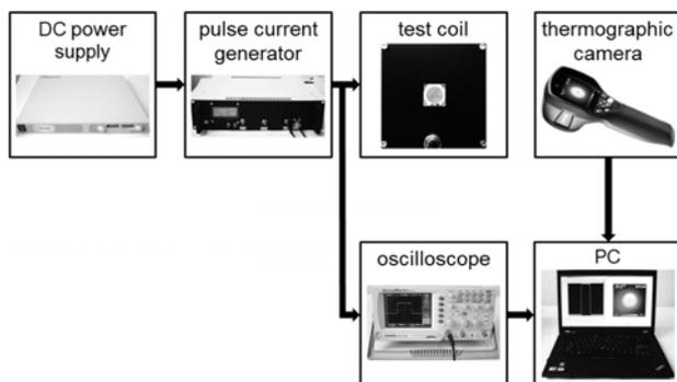
Fig.3. Block diagram of the measurement system
