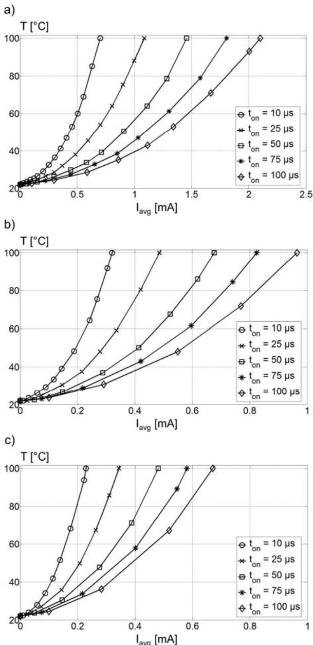
Fig.6. Temperature of the excitation coil as function of average value of current pulse for frequency: a) 1 Hz, b) 5 Hz, c) 10 Hz
