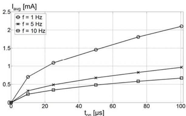
Fig.7. Average value of pulse current as function of duration time of the pulse current; temperature of the copper trace was equal to 100 °C
