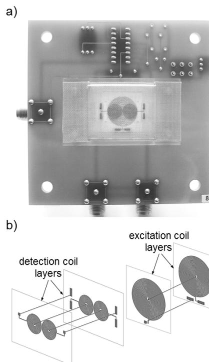
Fig.1. PCB transducer: a) photo, b) schematic view
