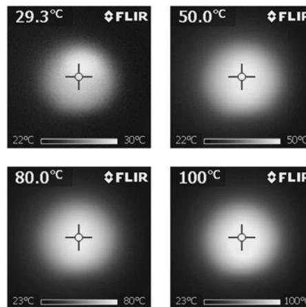
Fig.5. Thermal images of the test coil obtained during experiments
