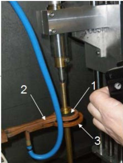
Fig. 6. Experimental stand 1 – gear wheel, 2 – inductor with connections, 3 - sprayer
