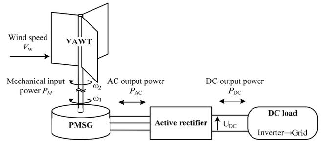
Fig.1. Function scheme of WECS
