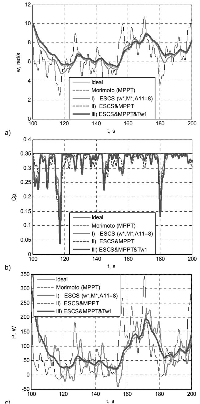
Fig.3. Time dependences of WECS operation with different control systems at  $V_{w,\text{mid}} = 4 \text{ m/s}$ : a) the VAWT angular speed; b) the wind power conversion efficiency factor; c) power, obtained from the generator during the fragment of the experimental period
