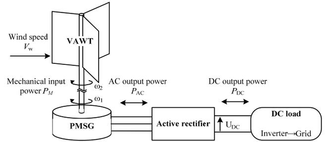
Fig.1. Function scheme of WECS
