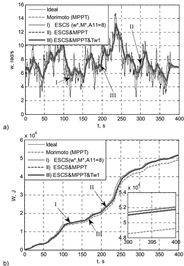
Fig.2. Time dependences of WECS operation with different control systems at  $V_{w,\text{mid}} = 4 \text{ m/s}$ : a) the PMSG angular speed, b) energy obtained from the generator during the experimental period
