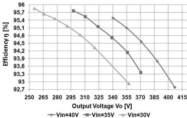
Fig.9. Efficiency  $\eta$  versus output voltage  $V_o$  for three different input voltages  $V_{in}=30$  V, 35 V, 40 V for different duty cycle  $D$  from 0.54 to 0.68
