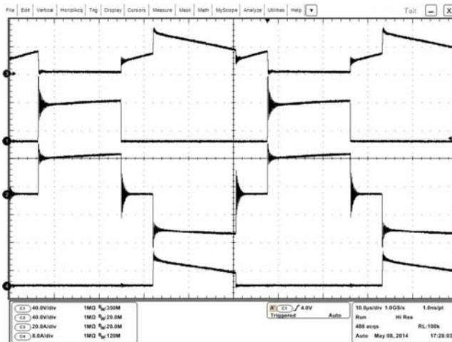
Fig.5. Measured waveforms of ch1-transistor  $S_1$  current  $i_{S1}$ , ch2-transistor  $S_1$  drain-to-source voltage  $v_{DS1}$ , ch3-transformer  $T_2$  primary side voltage  $v_{T2}$ , ch4-diode  $D_2$  current  $i_{D2}$
