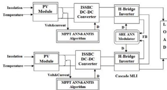
Fig.1. General Diagram of load connected photovoltaic system
