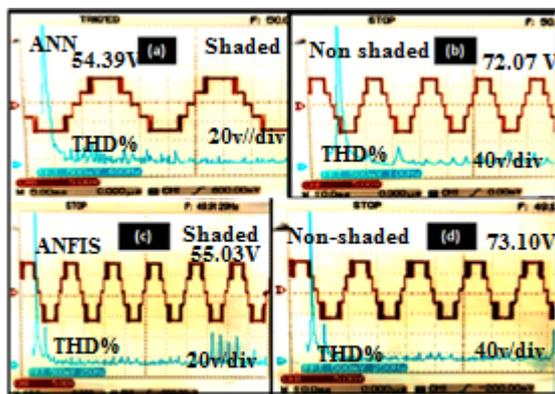
Fig.14.Experimental result for (a) shaded ANN output voltage and harmonic spectrum (b) Non-shaded ANN voltage harmonic spectrum (c) shaded ANFIS out voltage and harmonic spectrum (d) non-shaded ANN out voltage and harmonic spectrum
