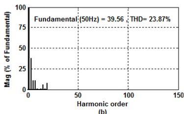
Fig.9.Simulation results for ANN MPPT under balanced condition (a) output voltage (b) voltage harmonic spectrum
