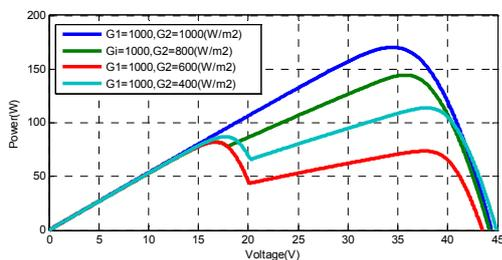
Fig. 6. P-V Curve at  $25^\circ\text{C}$
