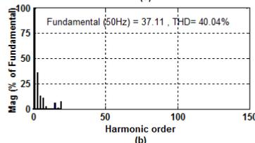
Fig.12.Simulation results for ANFIS MPPT under unbalanced condition (a) output voltage (b) voltage harmonic spectrum
