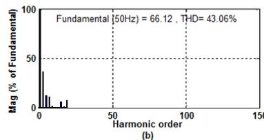
Fig.11.Simulation results for ANN MPPT under unbalanced condition (a) output voltage (b) voltage harmonic spectrum
