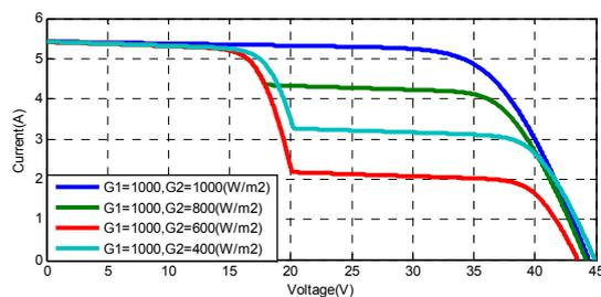
Fig. 7. I-V Curve at  $25^\circ\text{C}$
