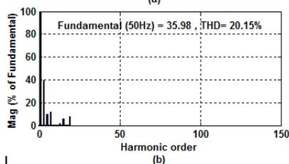
Fig.10 Simulation results for ANFIS MPPT under balanced condition (a) output voltage (b) voltage harmonic spectrum
