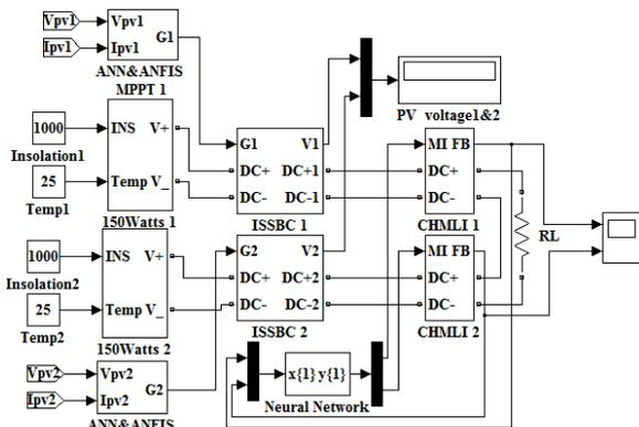
Fig.5. Simulation block diagram of the system
