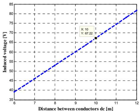
Fig.12. Variation of the induced voltage by varying the distance between conductors ( $h_c=12$  m)
