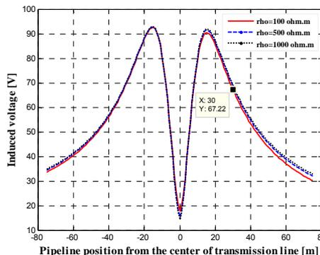
Fig.14. Variation of Induced voltage with the soil resistivity ( $d_p=30$  m,  $h_p=1$  m)
