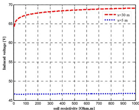
Fig.15. Relation between induced voltage and the soil resistivity ( $d_p=30$  m,  $d=5$  m,  $h_p=1$  m)
