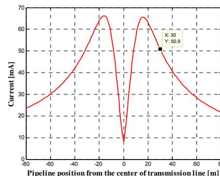
Fig.19. Shock current passing through the human body
