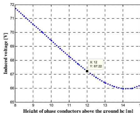
Fig.13. Variation of the induced voltage by varying the height of the conductors from the ground
