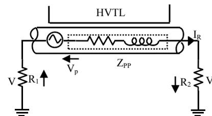
Fig.4. Pipeline and electrode resistance circuit
