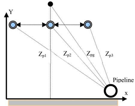
Fig.2. single-circuit overhead line with above pipeline
