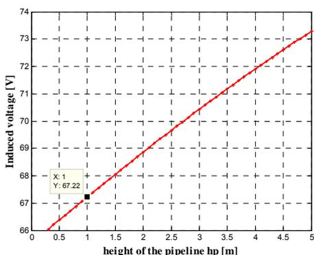
Fig.10. Relation between the induced voltage and the height of the pipeline ( $x_p=30$  m)
