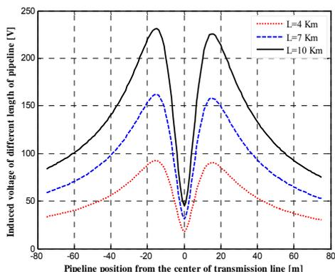
Fig.16. Variation of Induced voltage with the length of parallelism ( $d_p=30$  m,  $h_p=1$  m)
