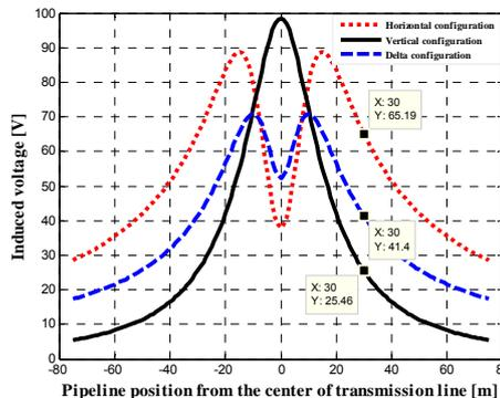
Fig.18. Induced voltage on the pipeline for various phase configurations
