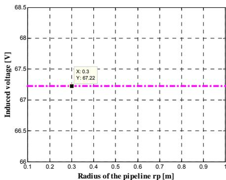
Fig.11. Relation between the induced voltage and the radius of the pipeline ( $d_p=30$  m,  $h_p=1$  m)
