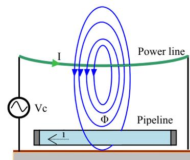
Fig.1. Inductive coupling between a pipeline and a power line
