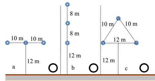
Fig.7. Different geometrical configurations for transmission overhead lines (a) horizontal, (b) vertical, (c) delta
