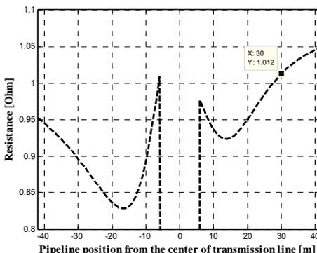
Fig.21. Earth electrode resistance of the pipeline
