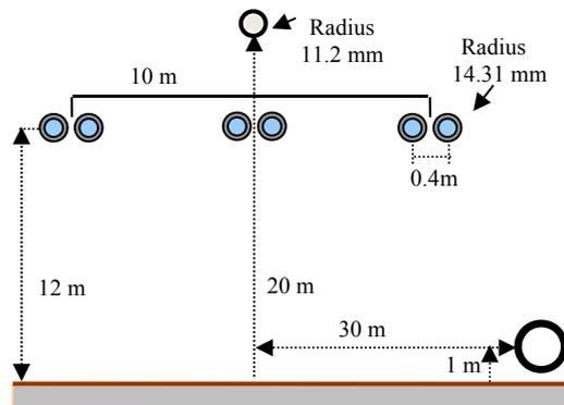
Fig.6. Single circuit horizontal configuration with ground wire and above pipeline
