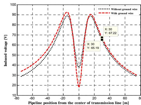
Fig.8. Induced voltage profile on the pipeline with and without the ground wire ( $d_p=30$  m,  $h_p=1$  m)
