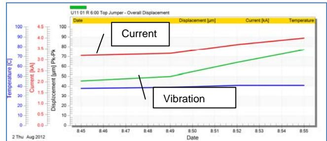
Fig. 3. Increasing Vibration with Current Trend
