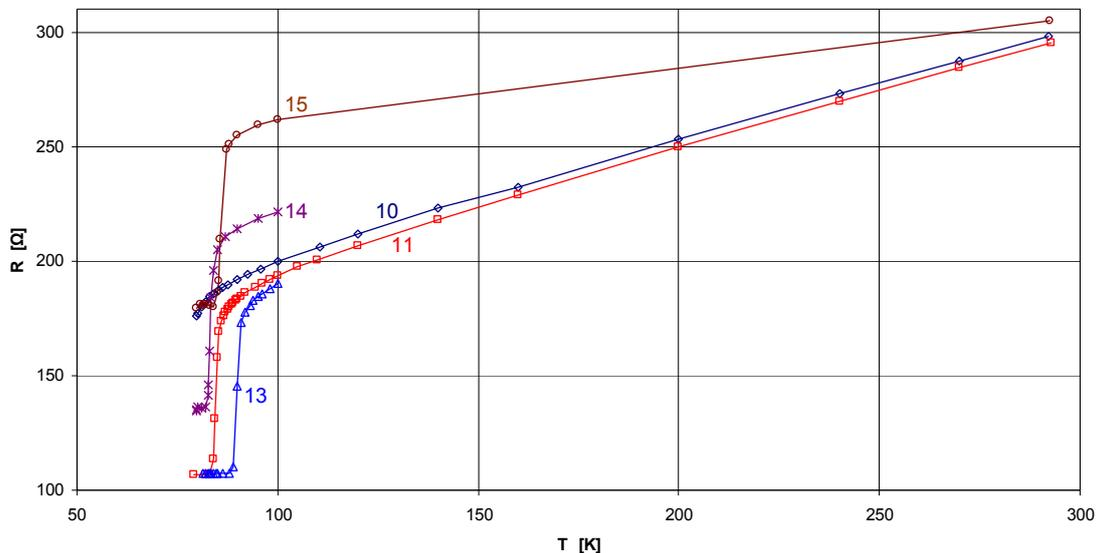
Fig. 3. Temperature dependences of the  $\text{YBa}_2\text{Cu}_3\text{O}_{7-x}$  microbridge resistance. The numbers of curves correspond with the order of carried out measurements.
