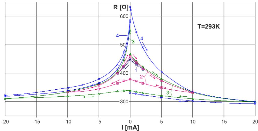
Fig.1 Resistance characteristics of an HTS microbridge in the room temperature under influence of a sequence of current cycles. The sequence of measurements corresponds with the numbers of curves and the direction of their arrows.
