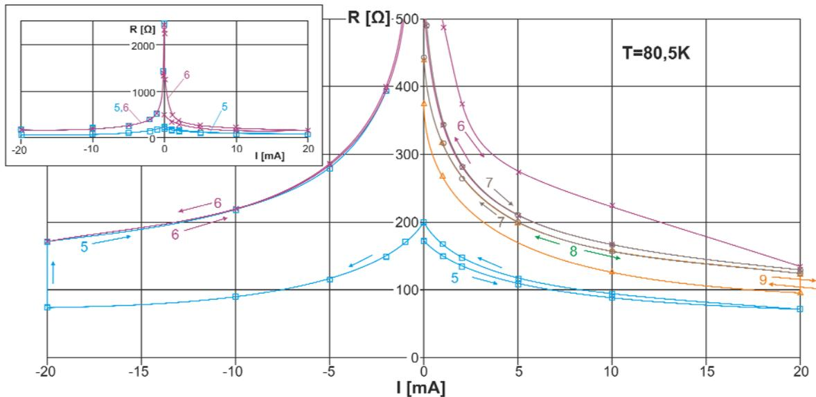
Fig. 2. Resistance characteristics of an HTS microbridge in the liquid nitrogen temperature under influence of a sequence of current cycles. The sequence of measurements corresponds with the numbers of curves and the direction of their arrows. In the insert – full 5 and 6 curves.
