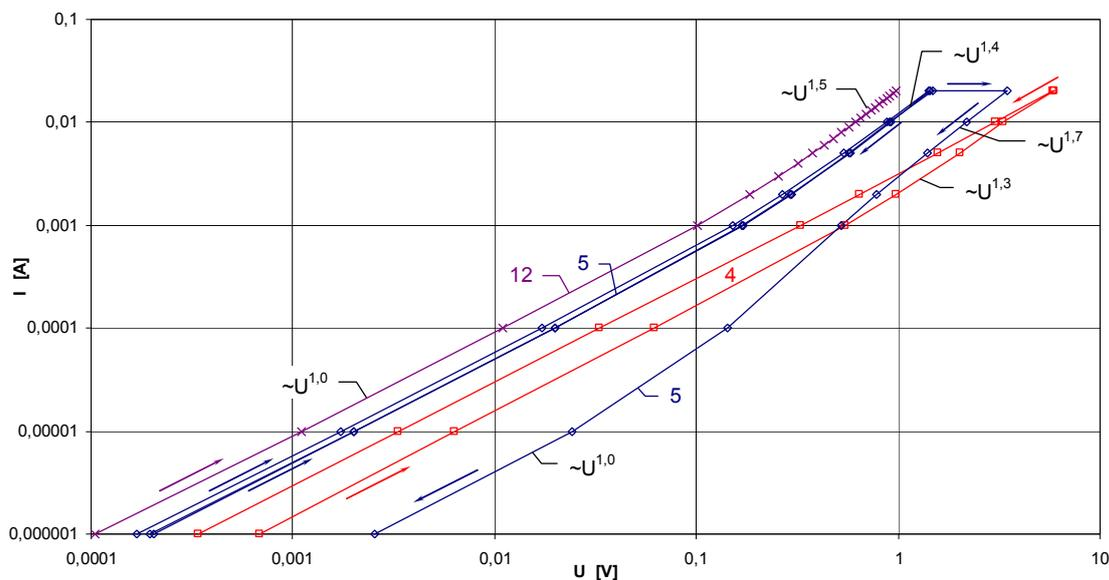
Fig. 4. Selected current-voltage characteristics of an HTS microbridge. The curves numbers correspond with Fig. 1 and 2. The arrows show the order of measurements (4 – when  $T=293K$ ; 5,12 – when  $T=80.5K$ ).
