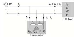
Fig. 4. Three-phase LTI load with reactive compensator
