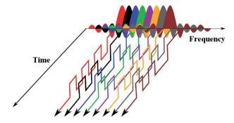
Fig.4. OFDM modulation [11]
