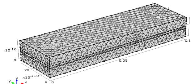
Fig. 3 Piezoelectric Shear Actuated Beam Mash.
