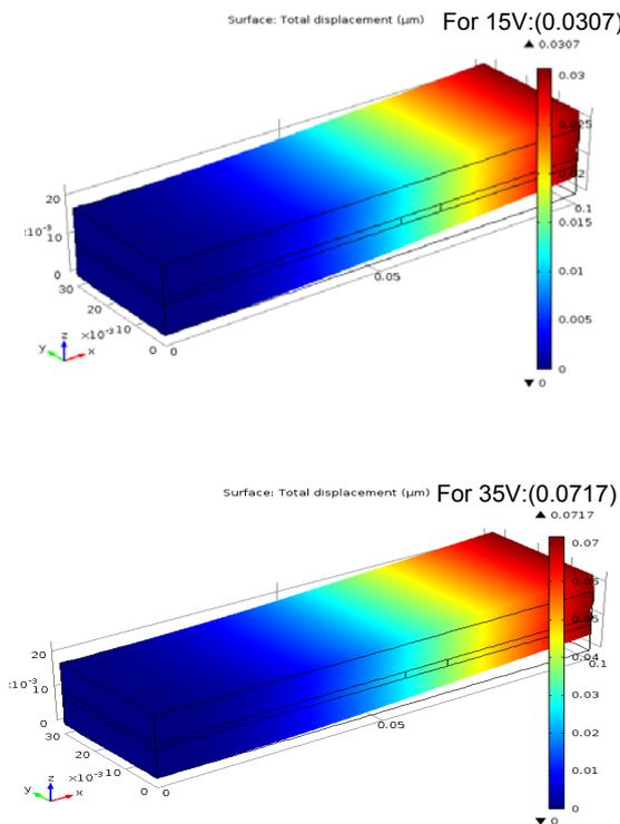
Fig. 5 Bend Beam plot for simulation-2.
