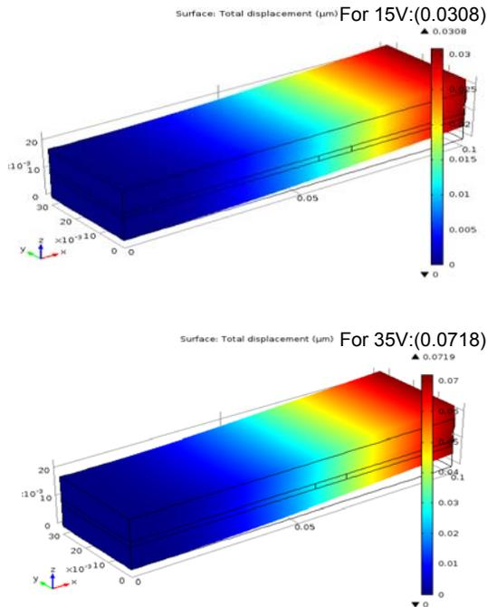
Fig. 4 Bend Beam plot for simulation-1
