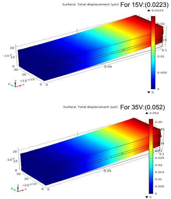
Fig. 6 Bend Beam plot for simulation-3.
