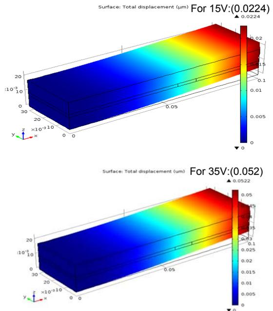
Fig. 7 Bend Beam plot for simulation-4.
