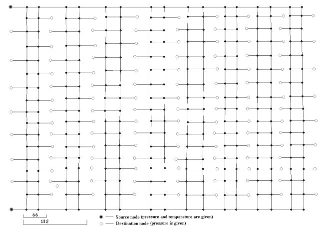
Fig. 1. The benchmark pipe network.
