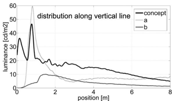
Fig.3. Luminance distributions along vertical line of symmetry
