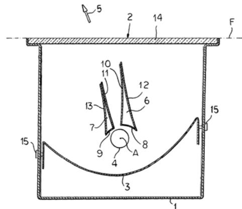
Fig.1. Cross-section drawing of luminaire "b" from patent document [10]
