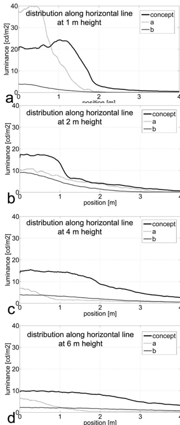
Fig.4. Luminance distributions along horizontal half lines
