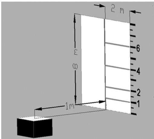
Fig.2. Lighting device geometry for simulations with indicated lines on the white test screen along which luminance distributions will be presented
