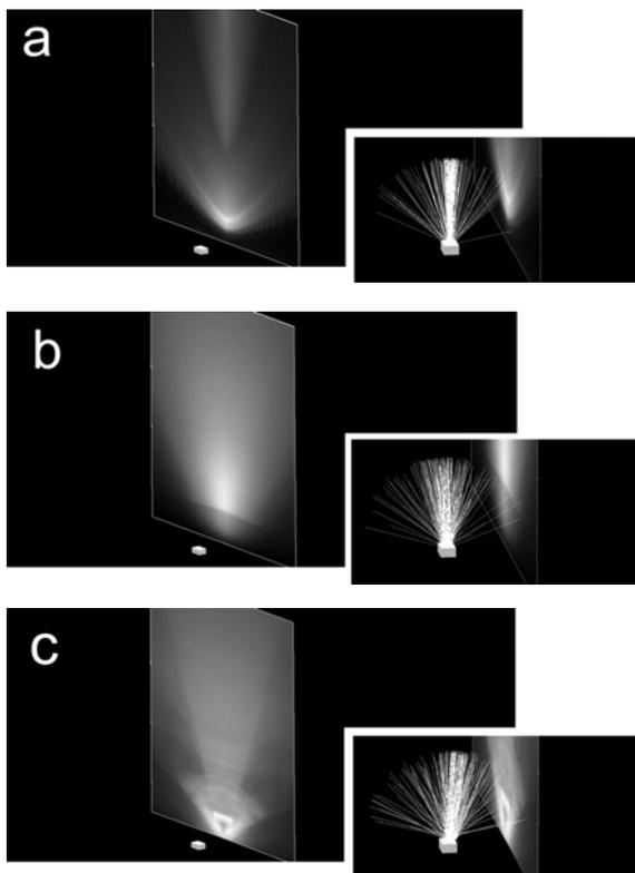
Fig.5. Visualizations of luminance distributions as a shaded plots (larger images) and rays emission visualizations (smaller images)
