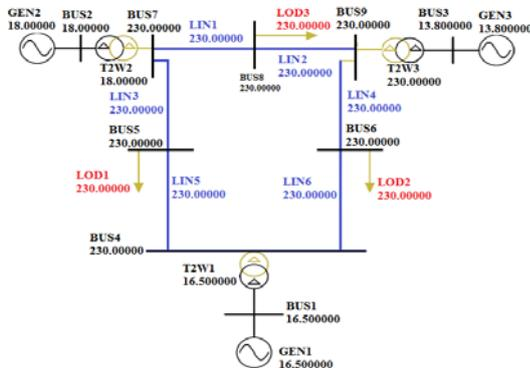
Fig.3. System IEEE, 9 Bus, with PowerApps.
