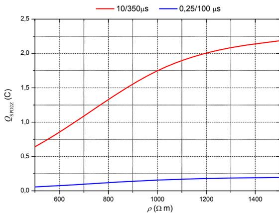
Fig.6. Charge  $Q_{SPD2z}$  associated to the current  $I_{SPD2}$  in a circuit with SPD at both ends for a meshed earth-termination system complying with IEC 62305-3; at lightning currents relevant to LPL I
