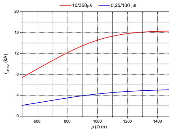
Fig.5. Current  $I_{SPD2z}$  in a circuit with SPD at both ends for a meshed earth-termination system complying with IEC 62305-3; at lightning currents relevant to LPL I
