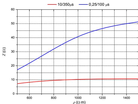
Fig.3. Conventional earth impedance  $Z$  as function of soil resistivity  $\rho$  for a meshed earth-termination system; at lightning currents relevant to LPL I
