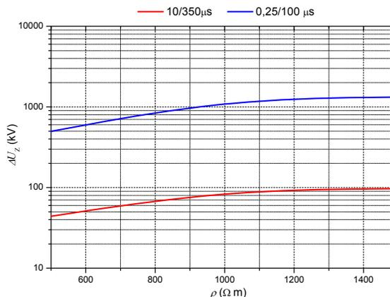
Fig.4. Voltage drop  $\Delta U_Z$  between the center and the edge of the grid complying with IEC 62305-3
