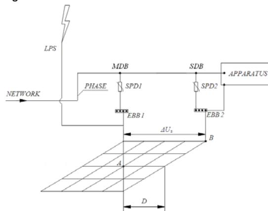
Fig.1. Diagram of circuit to supply an apparatus and the loop formed by phase conductors and two SPDs bonded to an extended earth arrangement (type B according to IEC/EN 62305-3) in different points
