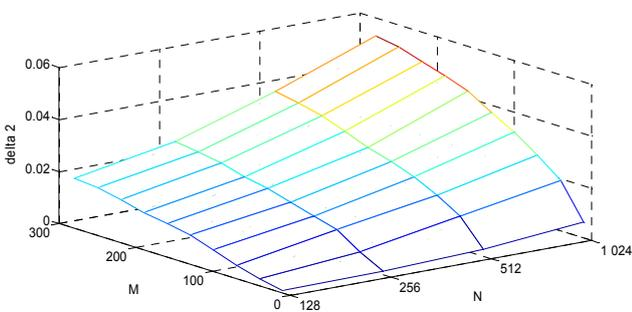
Fig. 5. A dependence of  $\delta_2$  on N and M for  $H_1(s)$ ,  $\delta_f = \delta_{Td} = 10^{-6}$
