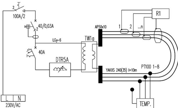
Fig. 1. The equivalent diagram of the laboratory stand
