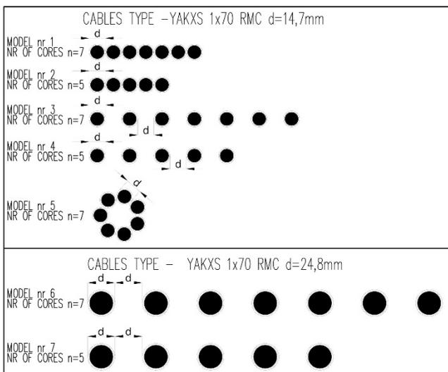
Fig. 2. Spatial configuration of the wires
