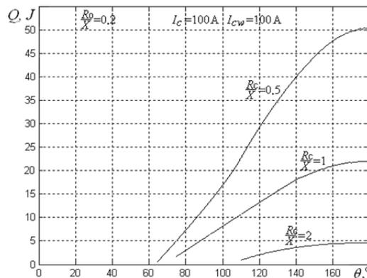
Fig. 10. Amount  $Q$  of heat as a function of angle  $\theta$  for selected values of the  $R/X$  ratio
