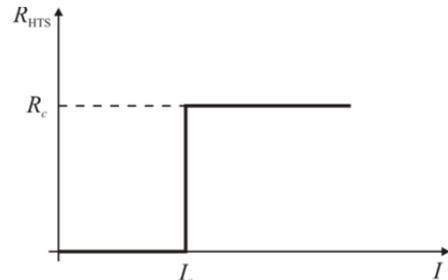
Fig. 5. Characteristics of HTS tape transition
