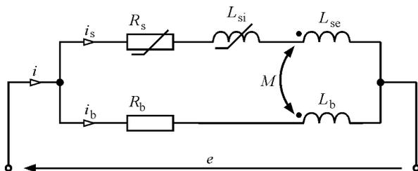
Fig. 4. The equivalent circuit of the superconducting tape [4]
