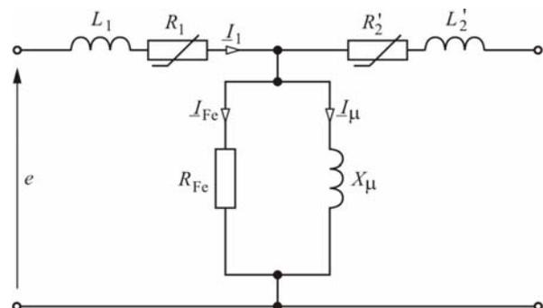
Fig. 2. The equivalent circuit of the superconducting transformer in an idle state
