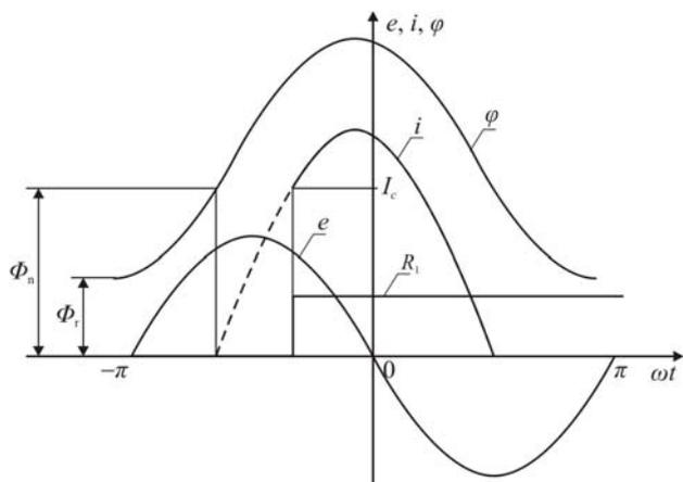
Fig. 7. Permanent loss of the superconducting state
