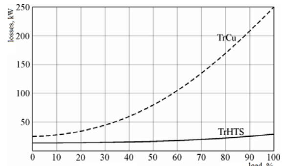
Fig. 1. Energy losses in transformers with HTS i Cu windings [2].
