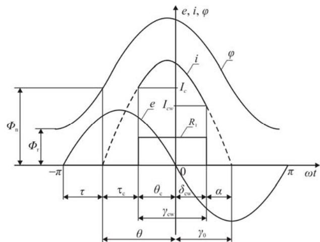
Fig. 6. Inrush current impulse
