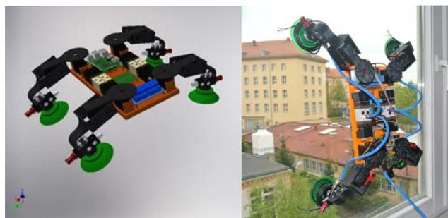
Fig.3. 3D visualization and photography of the Climbing Robot
