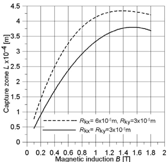
Fig.5. Width of the capture zone of the circular and elliptic collector's fibre versus the magnetic induction for paramagnetic particles at  $v_0 = 0.05$  m/s
