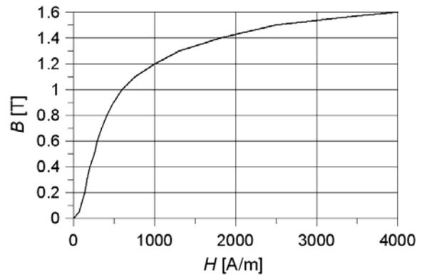
Fig.2. Magnetisation curve of the collector and particles
