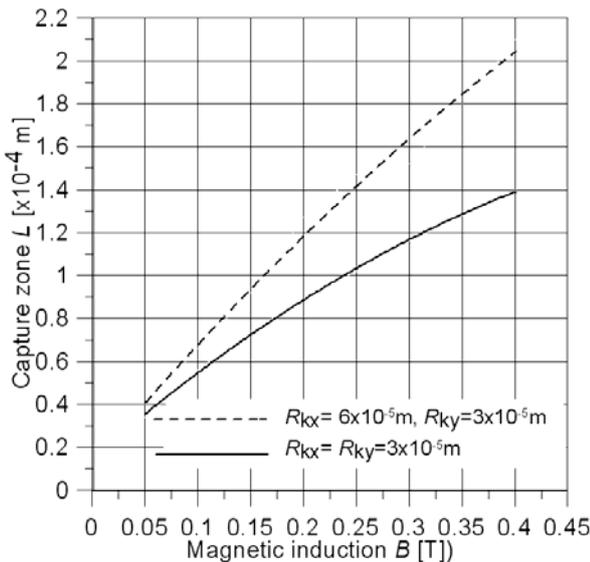
Fig.4. Width of the capture zone of the circular and elliptic collector's fibre versus the magnetic induction for ferromagnetic particles at  $v_0 = 0.05$  m/s
