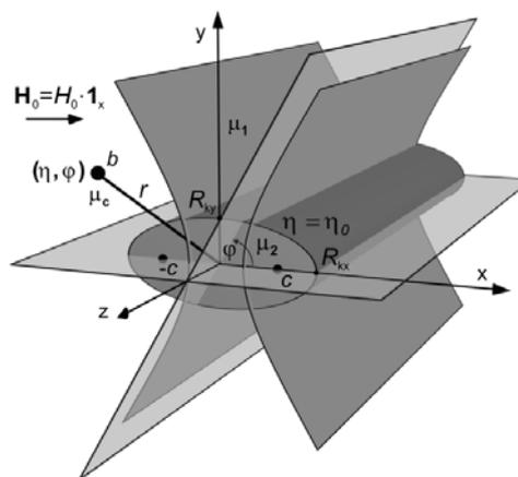
Fig.1. Elliptic cross-section collector and the particle placed in a homogeneous magnetic field
