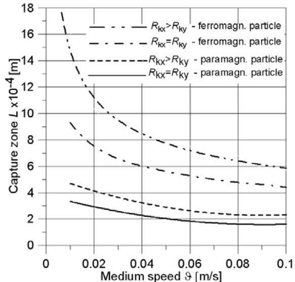
Fig.6. The dependence of the collector's capture zone on the speed of the medium flow carrying paramagnetic particles at the induction value  $B=0.5$  T, and ferromagnetic particles at the induction value  $B=0.1$  T for  $R_{kx} = R_{ky} = 3 \times 10^{-5}$  m and  $R_{kx} = 6 \times 10^{-5}$  m,  $R_{ky} = 3 \times 10^{-5}$  m
