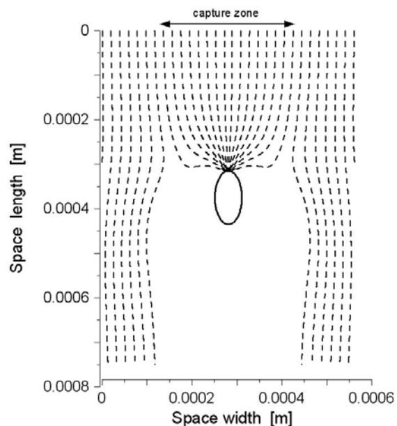
Fig.3. Trajectories of paramagnetic particles at magnetic induction  $B = 0.8$  T, radii of collector's section  $R_{ix} = 6 \cdot 10^{-5}$  m,  $R_{iy} = 3 \cdot 10^{-5}$  m
