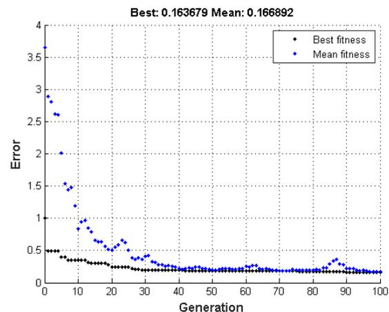
Fig. 8. The change of the objective function as a function of generations (the best individual and mean objective function of the population)
