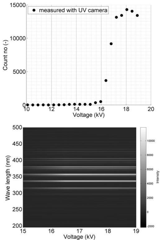
Fig. 2. Optical signals registered with the two considered methods on the cylindrical insulator
