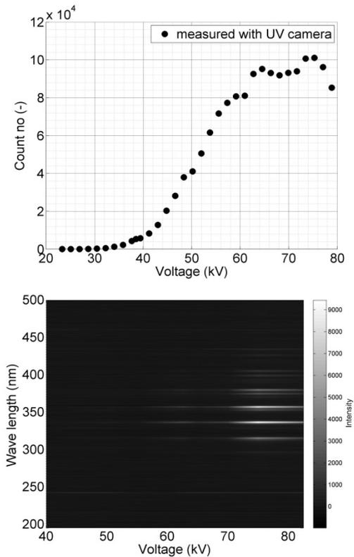
Fig.4. Optical signals registered with the two considered methods on the long rod insulator.
