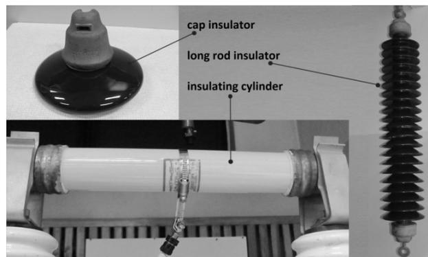
Fig.1. Pictures of the HV insulators applied in the study
