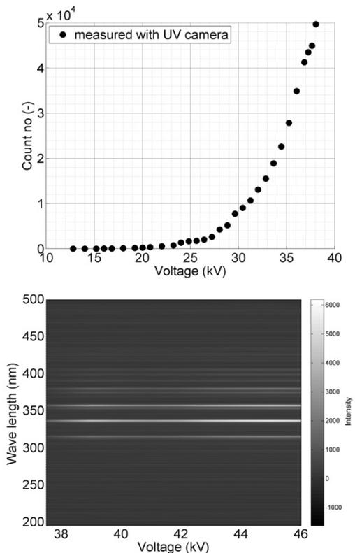
Fig.3. Optical signals registered with the two considered methods on the cap insulator
