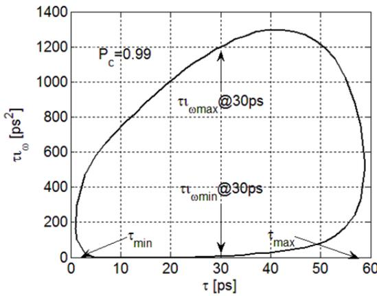
Fig.1. The contour delimiting the area with an arbitrary probability of  $[\tau, \tau_{\omega}]^T$  occurrence in a fiber with  $\tau_{av}=25ps$ .
