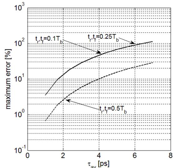
Fig.2. Confidence interval widths for errors of the DGD estimator versus average DGD in a fiber.
