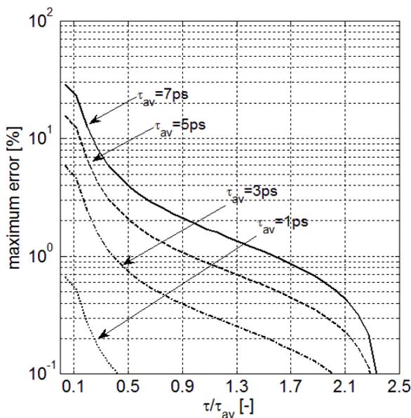
Fig.3. Confidence interval widths for errors of the DGD estimator versus ratio of momentary to average DGD.
