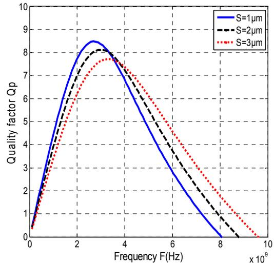
Fig. 12. Primary quality factor  $Q_p$  as a function of frequency and spacing between the traces  $S$  ( $1 \mu\text{m}$ ,  $2 \mu\text{m}$  and  $3 \mu\text{m}$ ).
