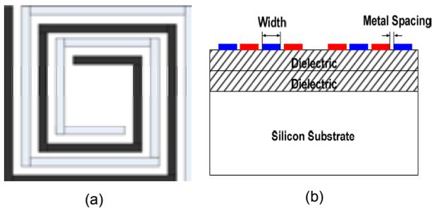
Fig. 3. (a) Top view of four-port interleaved transformer on silicon substrate. (b) Side view of interleaved transformer on silicon substrate.
