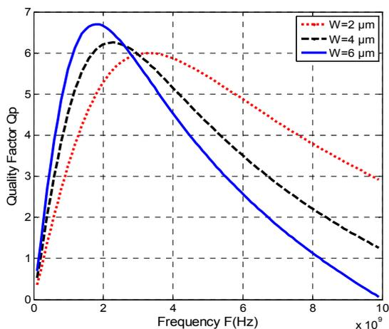
Fig. 10. Primary quality factor  $Q_p$  as a function of frequency and width of metal traces  $W$  ( $2 \mu\text{m}$ ,  $4 \mu\text{m}$  and  $6 \mu\text{m}$ ).
