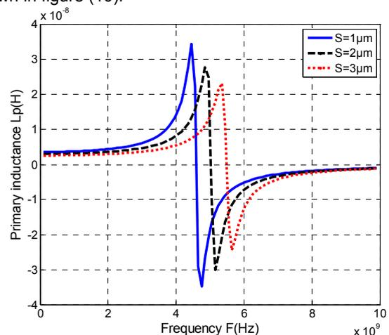
Fig. 11. Primary inductance  $L_p$  as a function of frequency and spacing between the traces  $S$  ( $1 \mu\text{m}$ ,  $2 \mu\text{m}$  and  $3 \mu\text{m}$ ).
