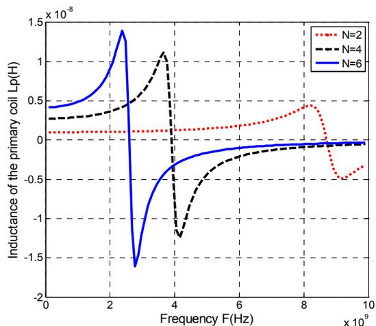
Fig.7. Primary inductance  $L_p$  as a function of frequency and number of turns  $N$  (2, 4 and 6).
