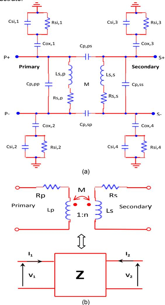
Fig. 4. (a) Compact equivalent circuit model of a silicon transformer, (b) Simplified model for transformer.
