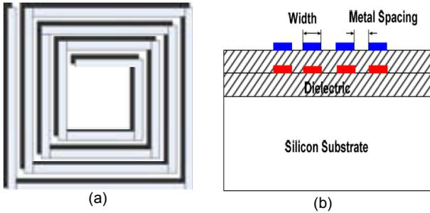
Fig. 2. (a) Top view of four-port stacked transformer on silicon substrate, (b) Side view of stacked transformer on silicon substrate.
