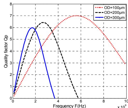
Fig. 6. Primary quality factor  $Q_p$  as a function of frequency and outer diameter  $OD$  (100 $\mu\text{m}$ , 200 $\mu\text{m}$  and 300 $\mu\text{m}$ ).
