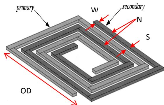
Fig. 1. Various geometrical parameter of the transformer.
