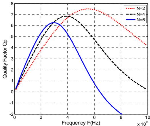
Fig.8. Primary quality factor  $Q_p$  as a function of frequency and number of turns  $N$  (2, 4 and 6).
