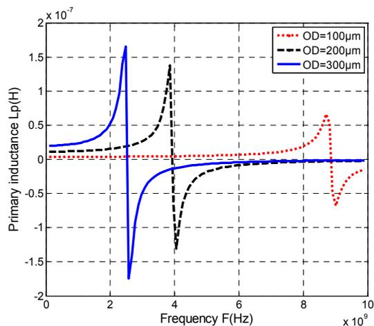
Fig.5. Primary inductance  $L_p$  as a function of frequency and outer diameter  $OD$  (100 $\mu\text{m}$ , 200 $\mu\text{m}$  and 300 $\mu\text{m}$ ).
