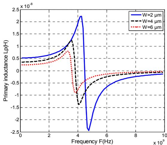
Fig.9. Primary inductance  $L_p$  as a function of frequency and width of metal traces  $W$  ( $2 \mu\text{m}$ ,  $4 \mu\text{m}$  and  $6 \mu\text{m}$ ).
