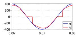
Fig. 7. Voltage waveform of the generator and voltage at the compensator location before compensation
