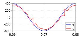
Fig. 8. Voltage waveform of the generator and voltage at the compensator location after compensation
