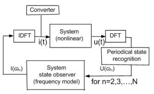
Fig. 2. Block diagram for searching of reference signal i(t)
