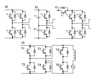
Fig. 5. Example of popular inverters: full-bridge (a), half-bridge (b), 5T bridge (c) and HERIC inverter (d)
