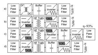
Fig. 8. Different variants of inverters topology for PV installations with HF transformers
