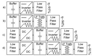
Fig. 3. Different solutions of PV inverters without transformer (a, b) and with LF transformer (c, d).
