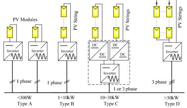
Fig. 1. Grid-connected PV systems: module inverter (Type A), string inverter (Type B), multi-string inverter (Type C) and central inverter (Type D).
