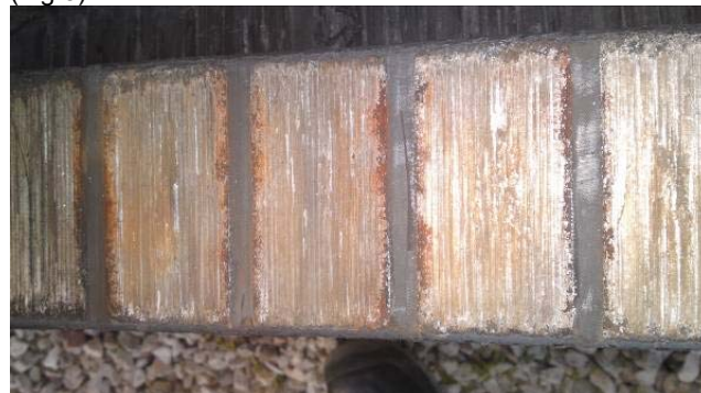
Fig. 5. Damage of stator bar outer corona protection due to bar vibration.
