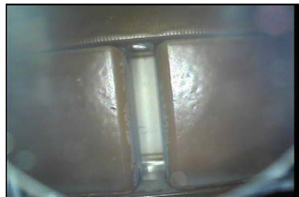
Fig. 10. Sample of visual inspection during LAI – movements in rotor wedges
