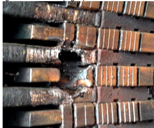
Fig. 2 Melted stator step iron due to very high temperature (high value of circulating current)
