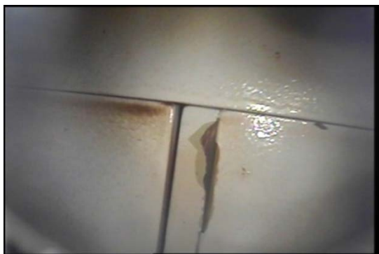
Fig. 11. Cracks of paint on rotor wedge - probably loose wedge
