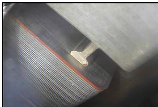
Fig. 15. Clean surface of air duct in middle part of the core
