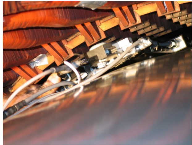
Fig. 8. RIV entering air-gap (150MW)
