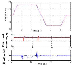
Fig.7 Simulation results under load torque condition and  $R_r$  variation with sequence 2.
