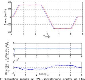
Fig.9: Simulation results of *RST*-Backstepping control at  $\pm 157$  *rad/sec* under load torque with inertia moment of  $1.25^*J$ .
