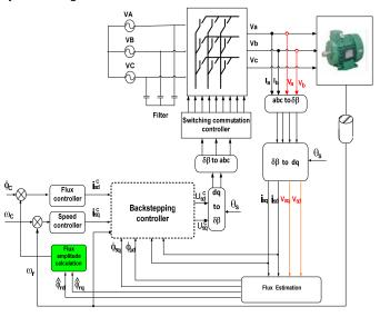
Fig. 3: *RST* speed control with nonlinear backstepping control scheme of *IM* motor.
