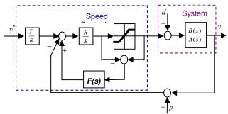
Fig.2: RST controller structure.
