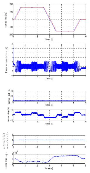
Fig.5: Sequence 2: Sensitivity of the performances system to change in the speed reference and load torque.
