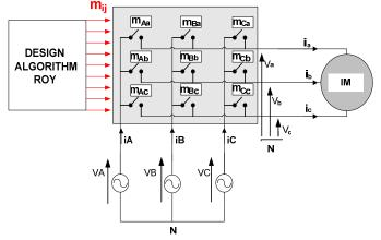
Fig.1: Circuit scheme of 3 phase to 3-phase matrix converter.
