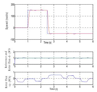
Fig. 8: Simulation results under load torque condition and J variation with sequence 1.
