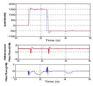
Fig.6 Simulation results under load torque condition and  $R_r$  variation with sequence 1.
