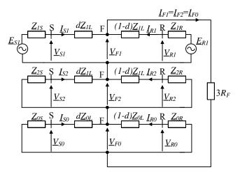
Fig. 2. Interconnection of equivalent networks for positive-, negative- and zero-sequence components under L1-E fault
